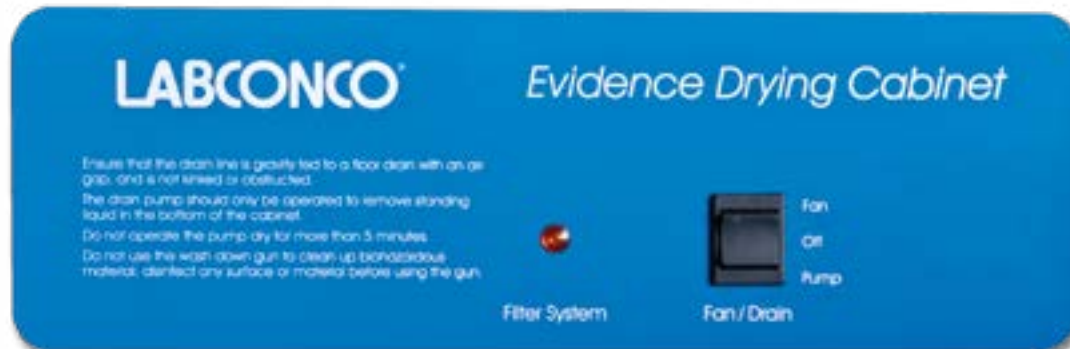
Close up of the control panel shows the filter system light and three-position fan/off/pump switch.
