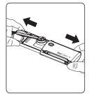
Once dried, the sample card can be removed from the EasiCollect+ and sent to the laboratory. Wearing gloves, hold the EasiCollect+ as shown and slide the cover open releasing the foam head.
